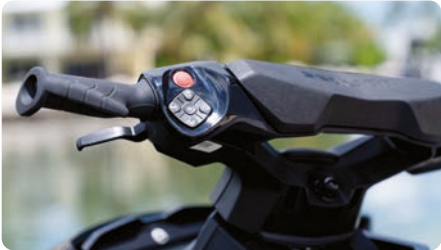
iDF - Intelligent Debris Free system An innovative, industry-first system that allows you to free your pump of weeds and debris with intuitive handlebar-activated controls.
